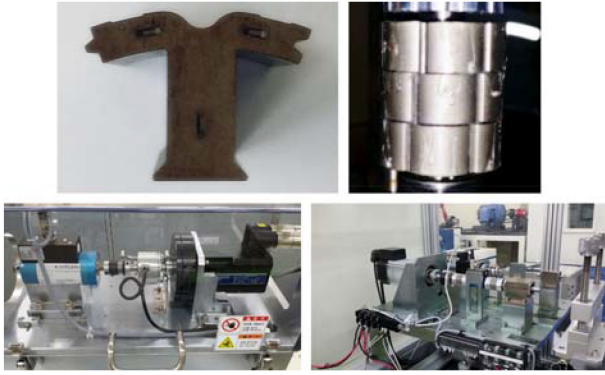
Fig. 1. Fabricated prototypes of SPMSM and measuring equipment [8].
