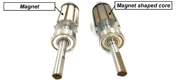
Fig. 10 Original rotor (left) with surface mounted magnet and rotor for iron loss separation (right) with magnet shaped core
