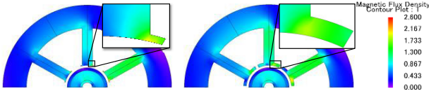
Fig. 7. Magnetic flux density contour of 2p6s one-slot pitch UHS PMSM according to slot opening width and tooth tip thickness.
