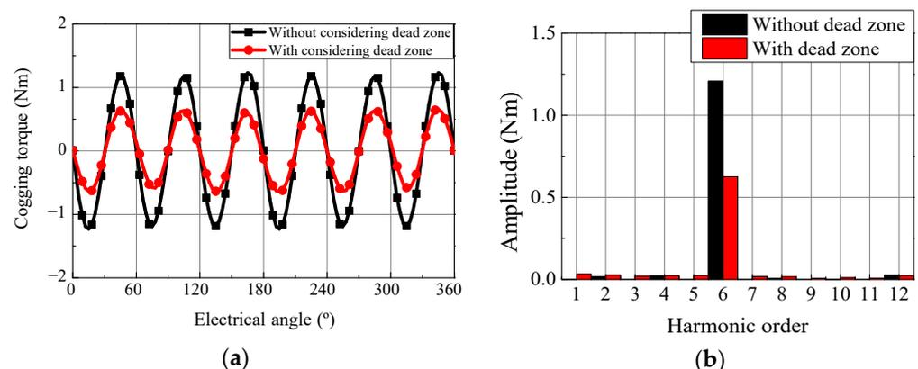
**Figure 2.** Cogging torque with/without dead zone. (a) Waveform; (b) harmonic analysis.
