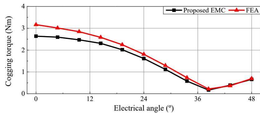
**Figure 9.** Cogging torque according to the dead zone angle.
