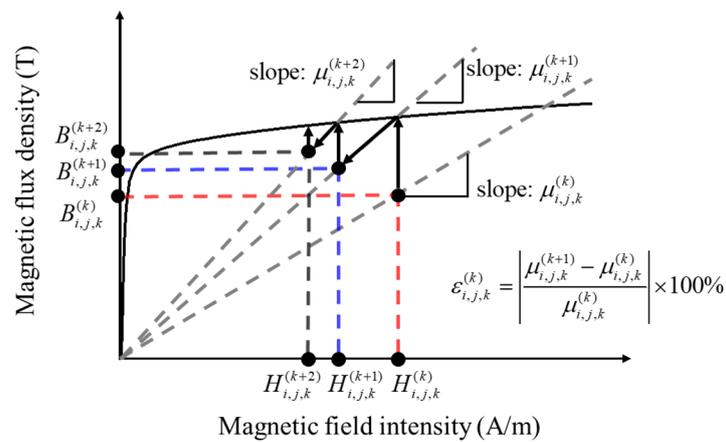
**Figure 4.** Nonlinear magnetizing curve and convergence process.
