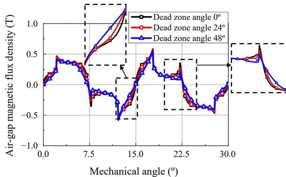
**Figure 6.** No-load radial air-gap magnetic flux density distribution calculated using the proposed EMC according to the dead zone angle.
