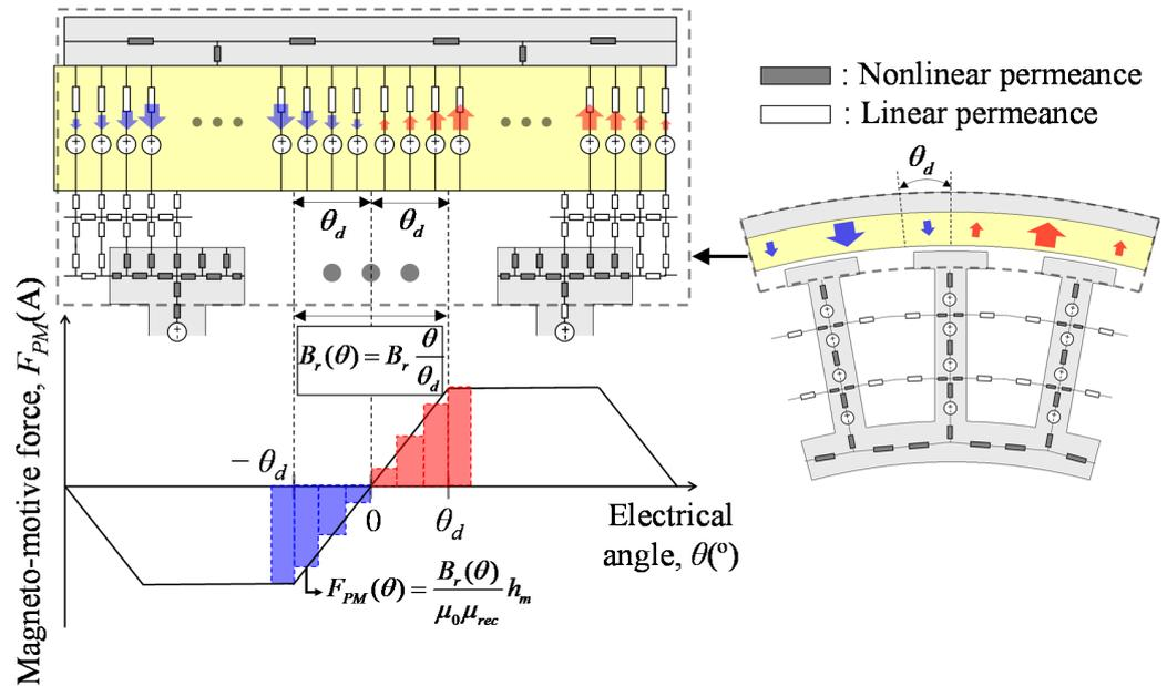
Figure 3. Equivalent magnetic circuit considering PM dead zone.
