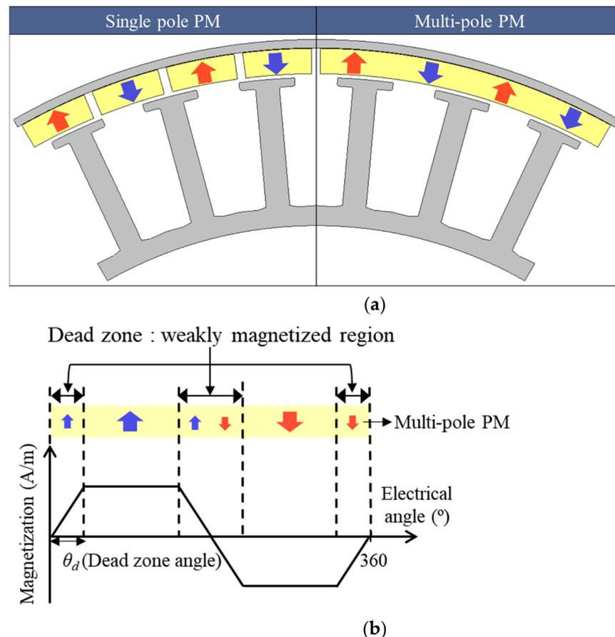
**Figure 1.** Motor with multi-pole PM: (a) Configuration; (b) magnetization distribution.
