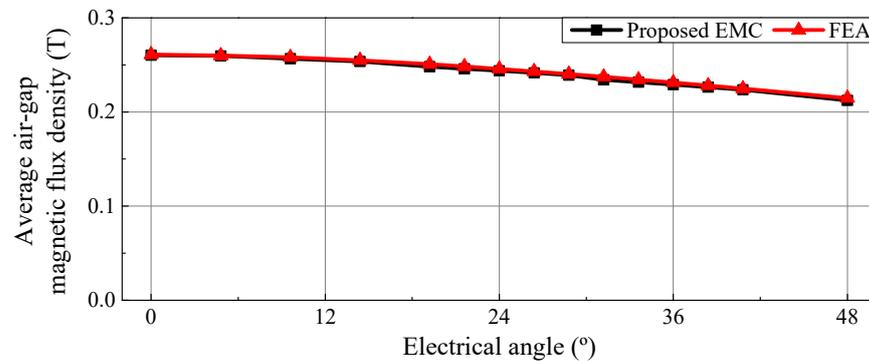
**Figure 8.** Average air-gap magnetic flux density according to the dead zone angle.
