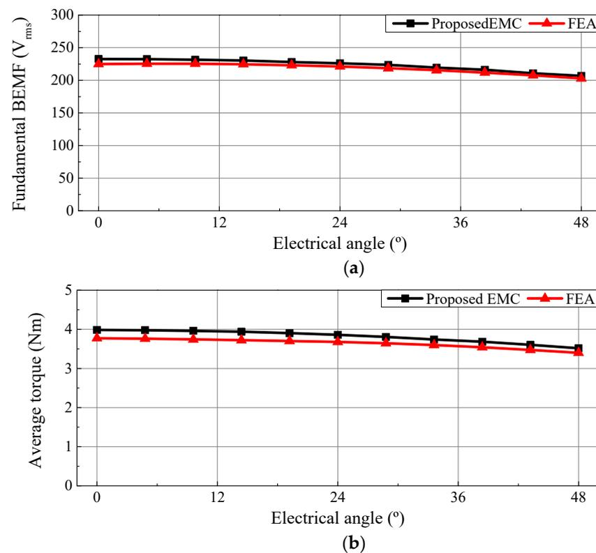
**Figure 10.** BEMF and average torque according to the dead zone angle. (a) Fundamental BEMF; (b) average torque.
