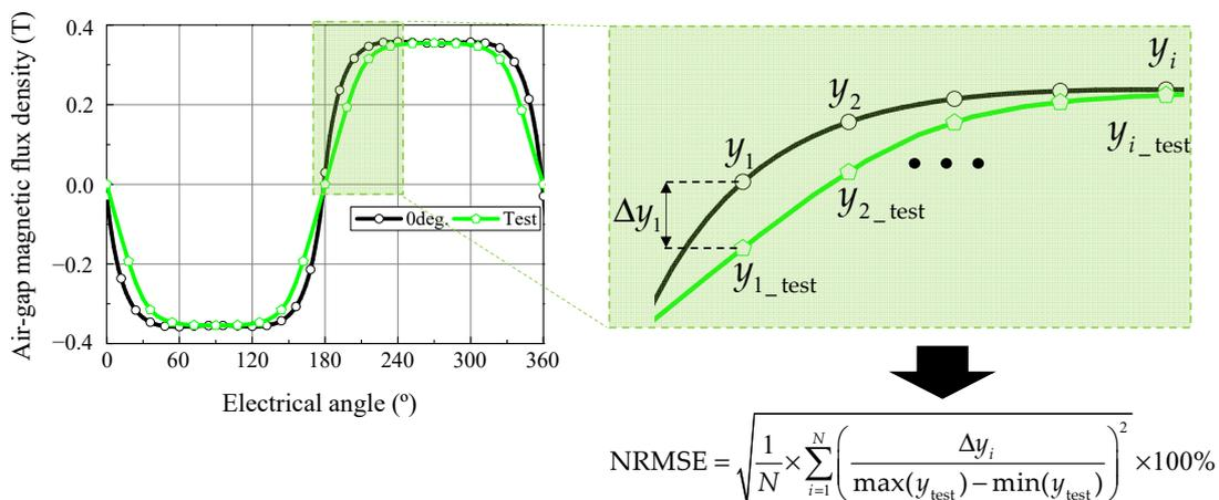
Figure 12. NRMSE calculation process.
