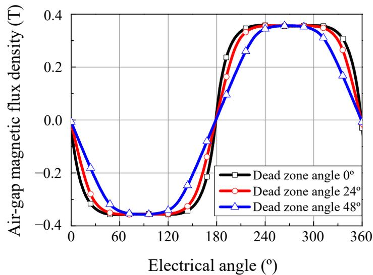
**Figure 7.** No-load air-gap magnetic flux density calculated using the proposed EMC according to the dead zone angle.
