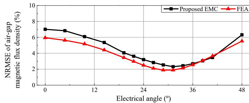
Figure 13. NRMSE of the air-gap magnetic flux density according to the dead zone angle.
