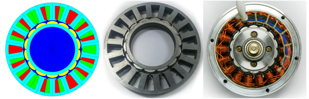
Fig. 14. Final model for the wearable robot joint; 2-D FEA model (left), manufactured sample (center and right).
