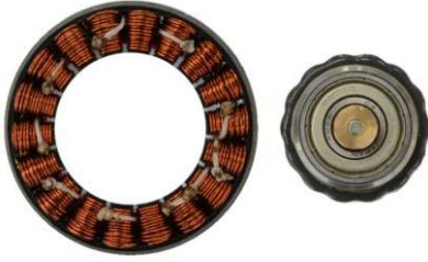
Fig. 4. SPMSM designed for exoskeleton wearable robots.
