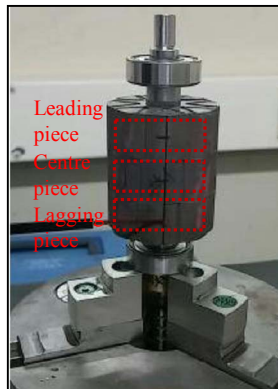
Fig. 8. Measurement of rotor surface flux density
