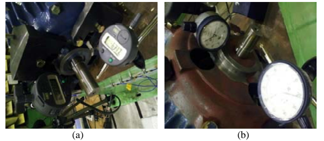
Fig. 6. Experimental setup for measuring the eccentricity: (a) dial gauge at the front part of the motor; and (b) dial gauge at the back part of the motor.
