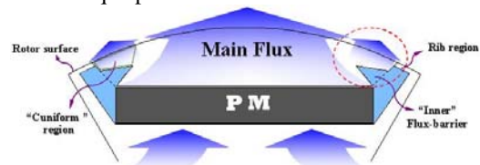
Fig. 3. Graphical illustration of magnetic flux distribution of novel design
