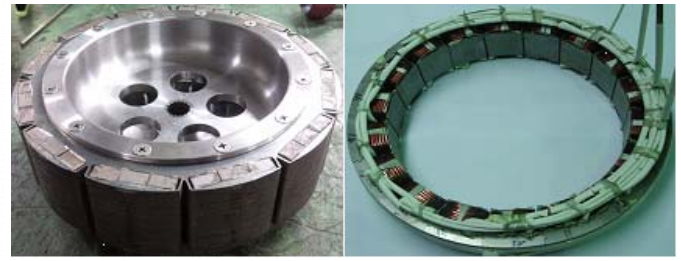
Fig. 10. Fabricated rotor and stator of in-wheel motor
