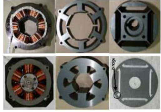
Fig. 8. Fabricated 4-pole/6-slot IPMSMs (ferrite and NdFeB magnet)
