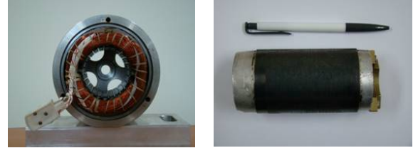
(a) Stator and rotor configuration of LSPMM
