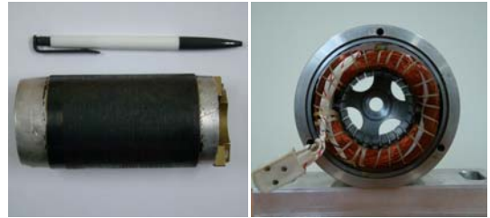
Fig. 9. Rotor and stator of improved LSPM motor
