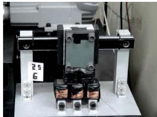
Figure 7: Proto linear oscillatory actuator
