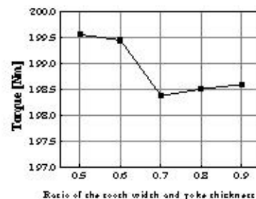
(c) 16 poles 24 slots Fig.7. Predicted the torque.
