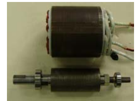
Fig. 7. The fabricated IPMSM
