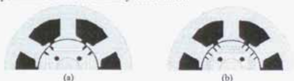
Fig 2. (a) Prototype single layer and (b) Re-designed double-layer IPMSM
