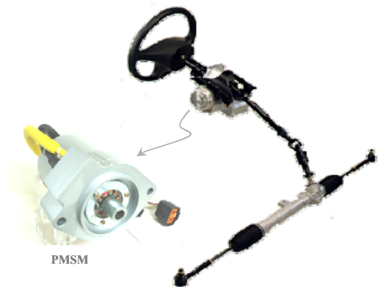
Fig.1. Column typed EPS system and PMSM
