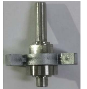
(B) Rotor and shaft
