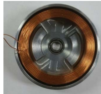
(A) Housing (lower stator) and coil wound
