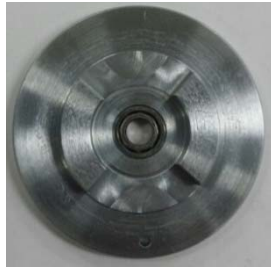
(C) Housing (upper stator)
